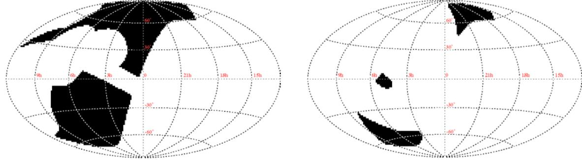
**Figure 2.** Visibility (dark region) for 3 January 2003. Left panel shows regions of stability for 1000 seconds; these regions shrink (right panel) if a day-long observation is desired.
