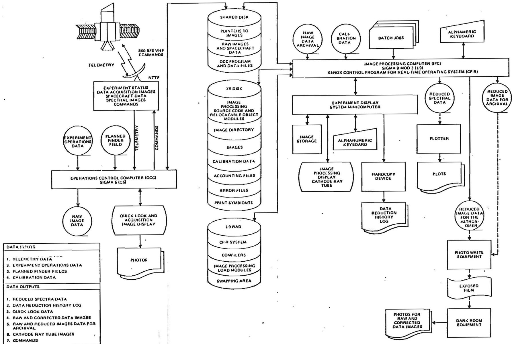
Figure 2-1. The International Ultraviolet Explorer (IUE) Image Processing Data Flow: Spacecraft to Astronomer
