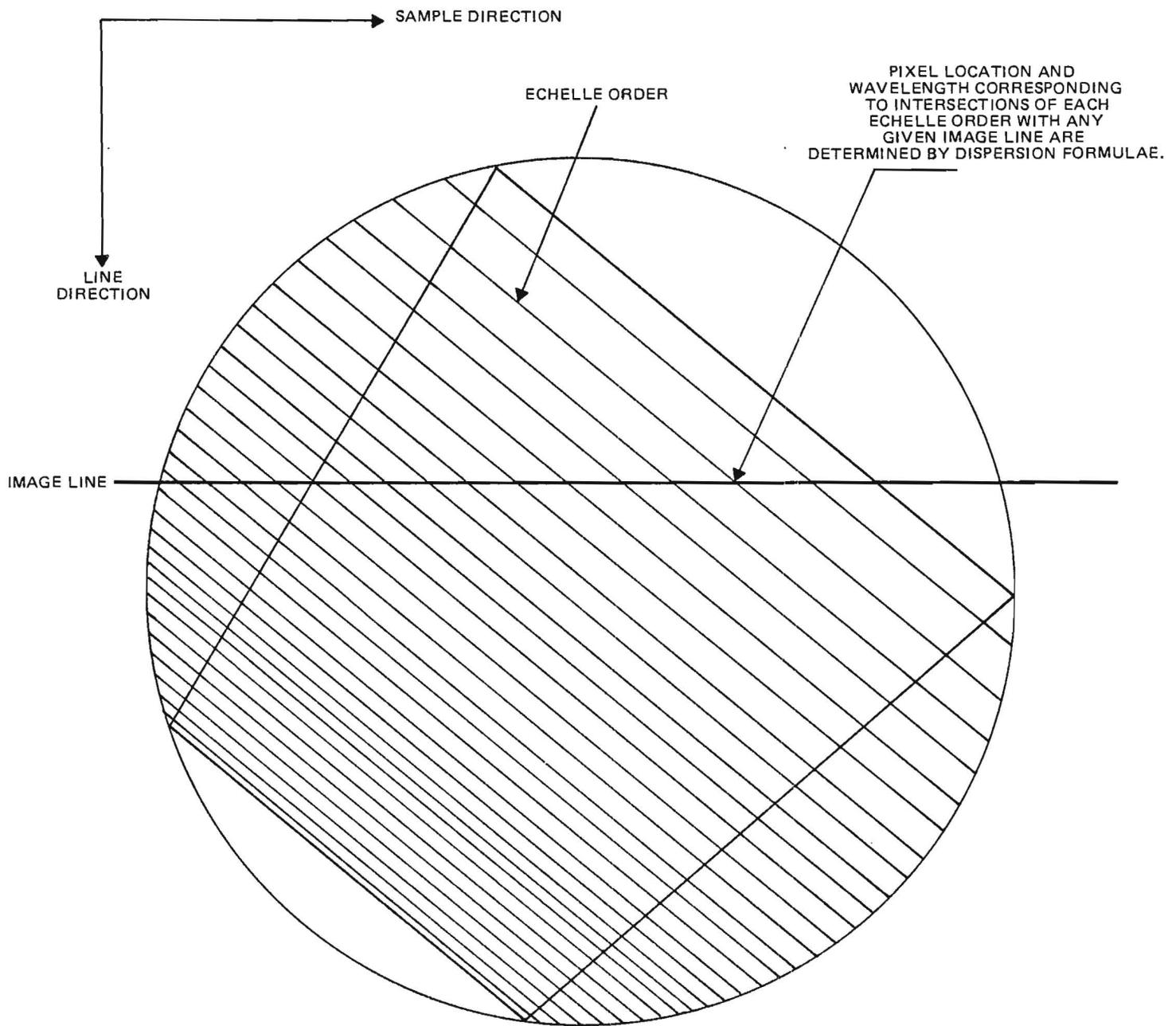
Figure 4-6. Schematic Echelle Image Format
