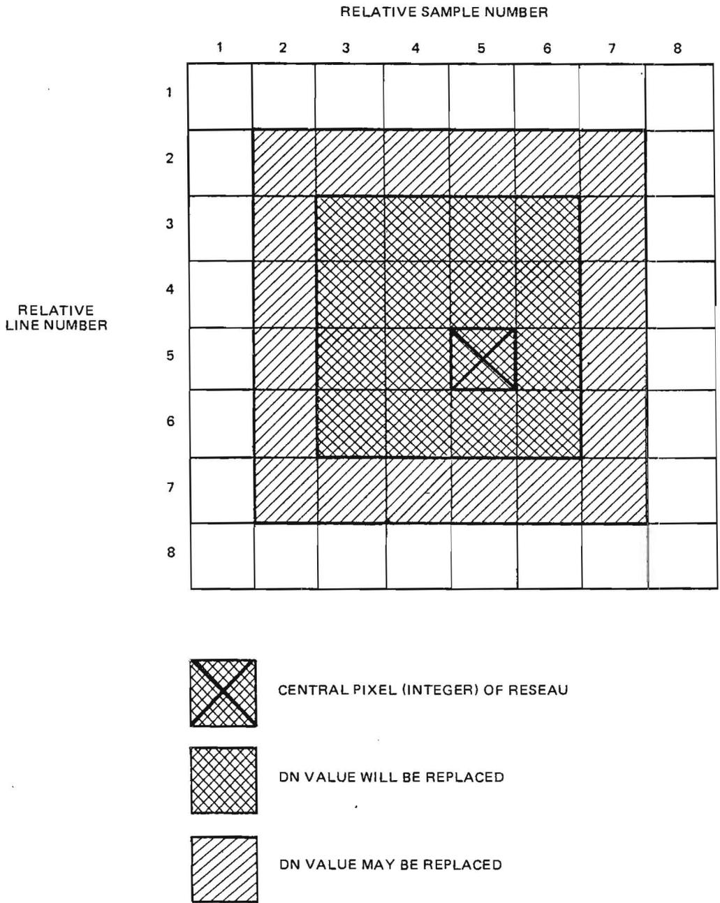
Figure 4-3. Pixel Array for Reseau Removal
