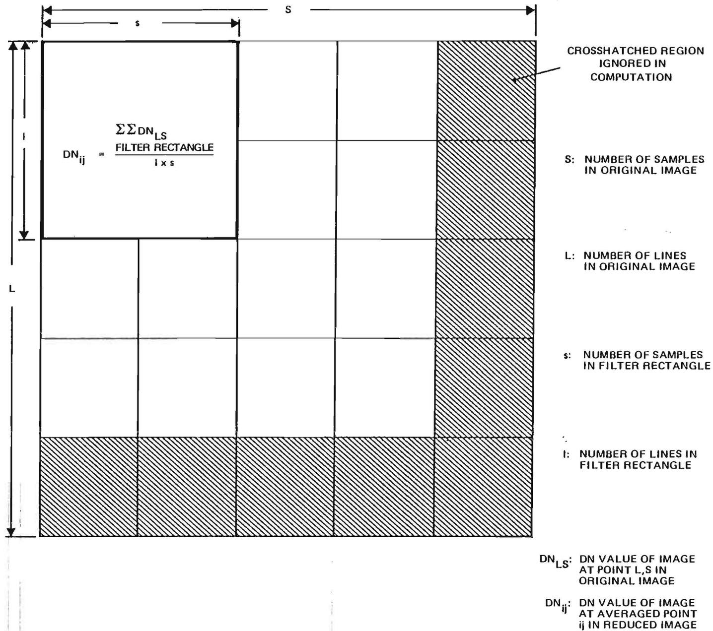
Figure 4-2. A Two-by-Two Pixel BOXAV Filter
