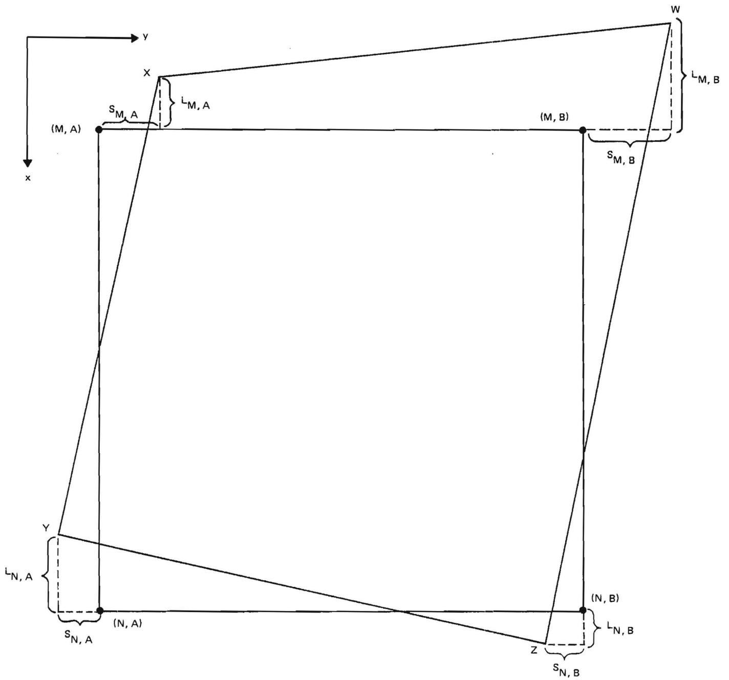
Figure 4-4. Geometric Distortion Displacements
