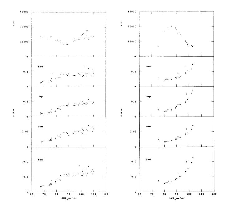
Figure 1. Noise characteristics of various regions of SWP (left) and LWP (right) cameras as functions of order number. From bottom to top: typical individual spectrum (ind), sum of 15 spectra (sum), template spectrum (tmp), and computed random noise in individual spectrum (rnd). At the top is the mean net flux.
