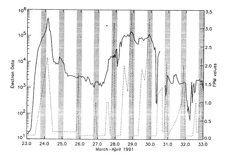
Figure 1: Data from the GOES-7 (solid) and IUE (dotted). US2 shift is shaded. The solar event of March 23-24, 1991 affected our radiation levels for several days. Initially suppressed, the FPM rose significantly on the 27th and the days that followed.
