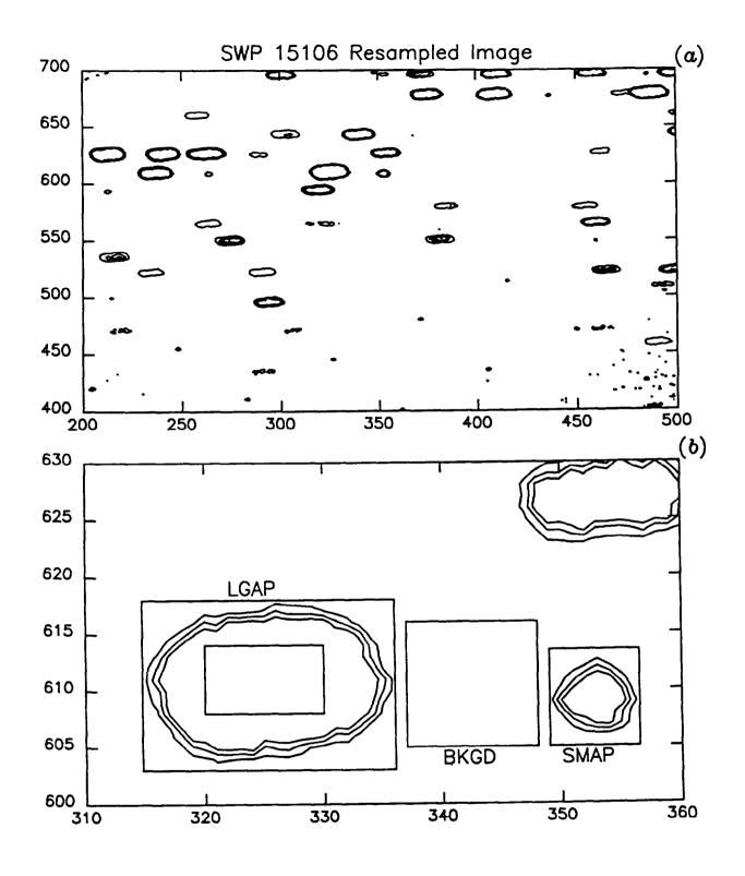
Figure 1: Panel a shows a section of the camera faceplate for a WAVECAL image. Panel b shows an expanded view of a small- and large- aperture Pt-Ne emission feature.
